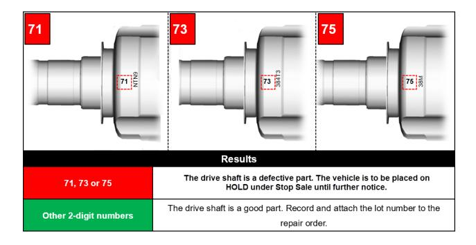
**STEP 4:** Do any of the drive shafts require replacement?
