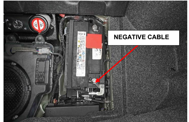
Figure 1 – Negative Battery Cable
