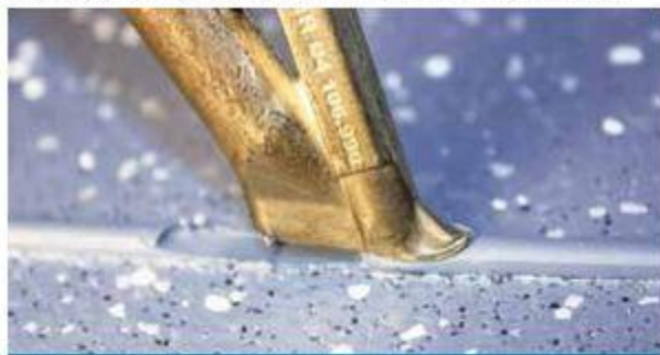
Overlapped weldrod in middle of seam
