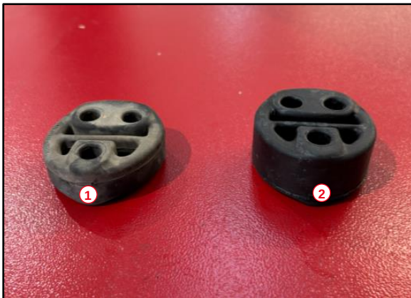
Figure 2. Exhaust Support Hanger 3
