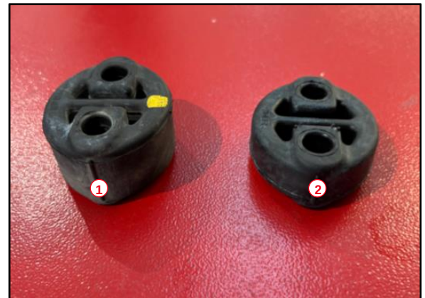
Figure 3. Exhaust Support Hanger 4
