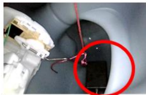
Figure 3: Fuel sender arm getting stuck against NG fuel tank. Unable to float to top "F".
