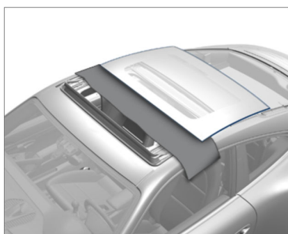
Fitting protective cover
