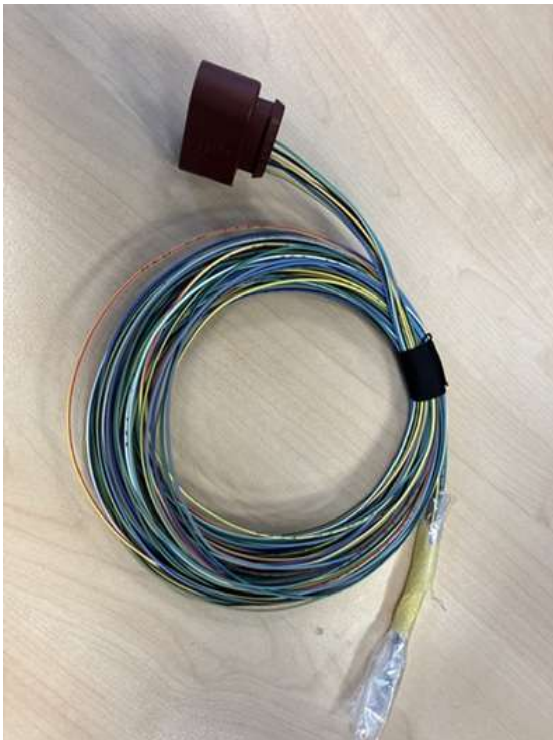
Figure 2. Wiring harness with part number 4P0971065 for Audi A5 (FU) and Audi A6 (FN)
