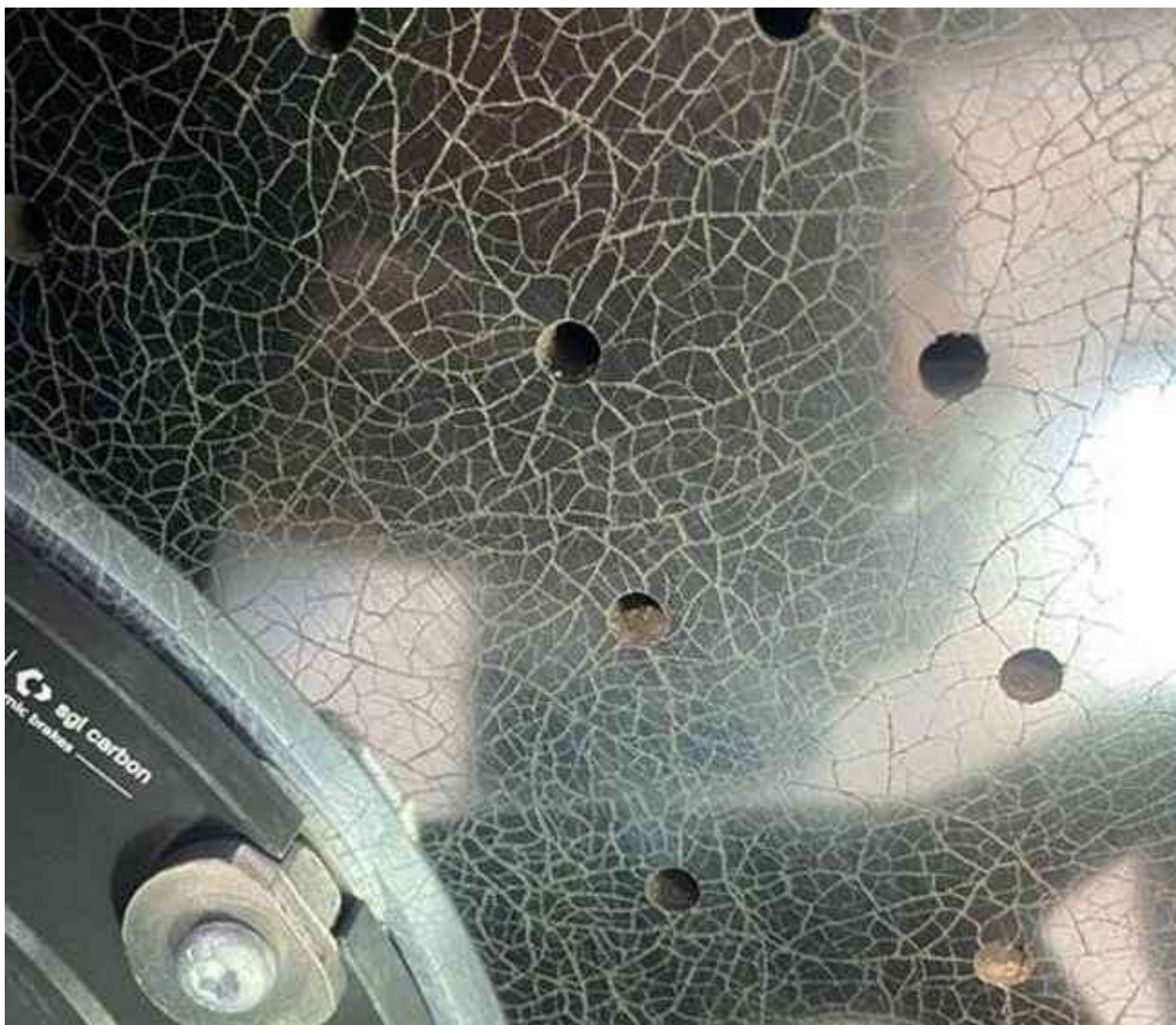
Figure 1. Cracks on the surface of the friction ring.
