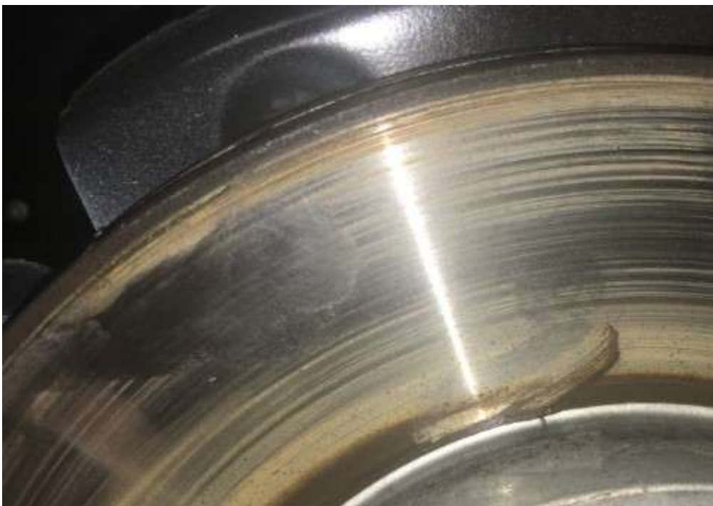
Figure 2: Example of a dirty friction surface on the brake disc.
