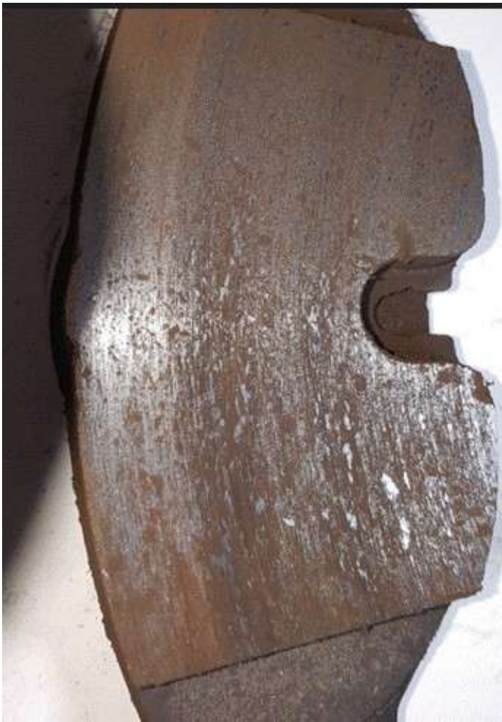
Figure 1: Example of a dirty friction surface on the brake pad.
