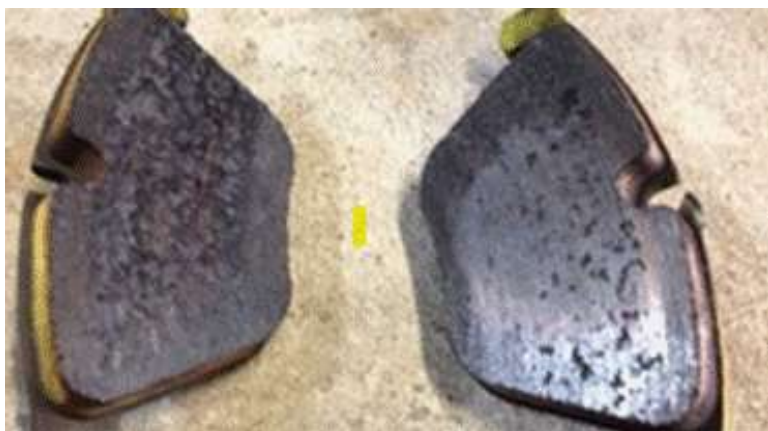
Figure 3: Example of brake pads with glazed friction surface.
