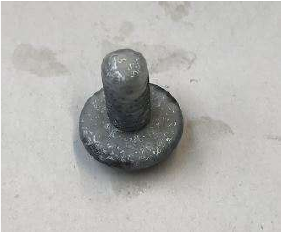
Figure 2. Securing bolt for splash plate for brake disc.
