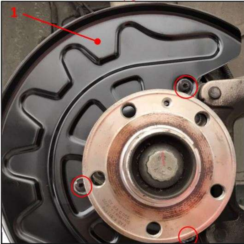
Figure 1. Splash plate for brake disc with contact surfaces of securing bolts.
