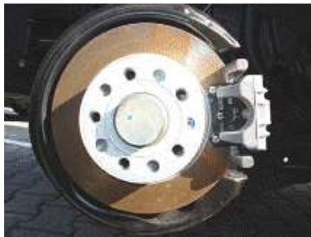
Figure 1: Example of excessively rusted disc brakes. Figure 2: Example of rusted disc brake surface.
