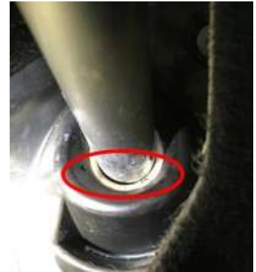
Figure 1. Poor sealing on the intermediate shaft.
