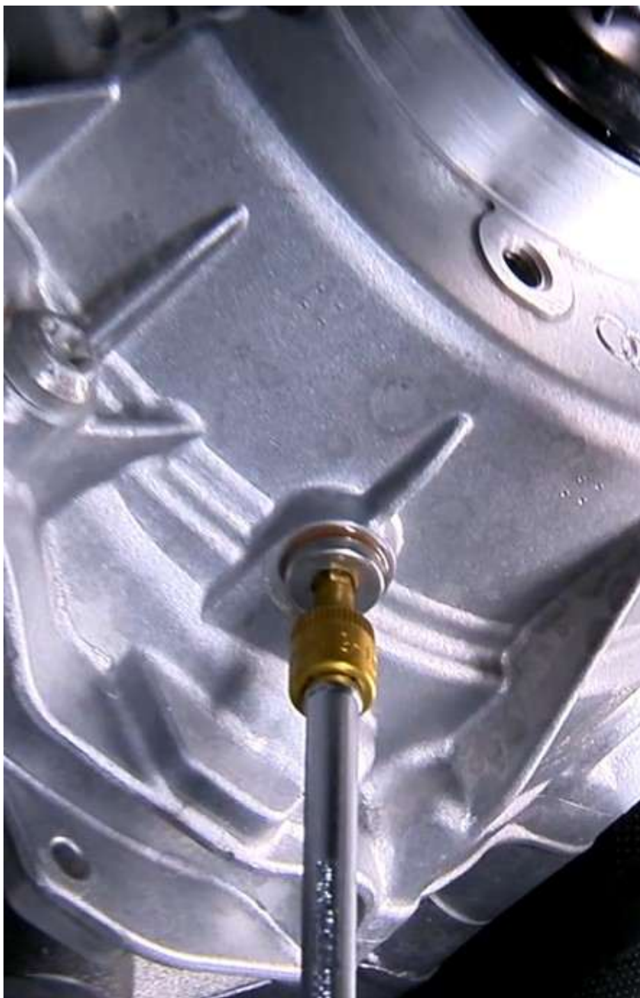
Figure 3. Tightening the drain plug.
