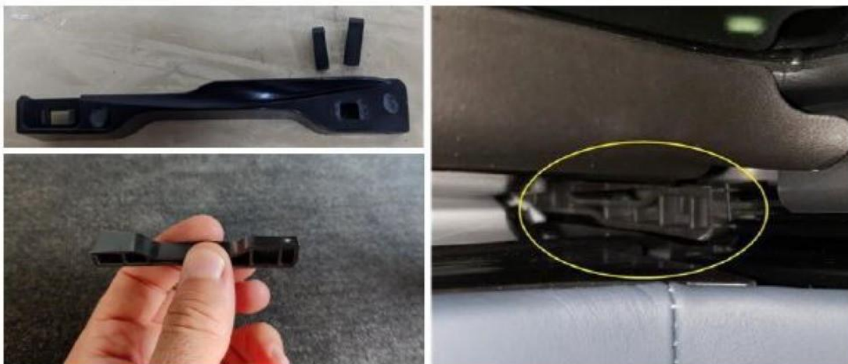
Figure 8 Examples of missing, loose and damaged guide parts
