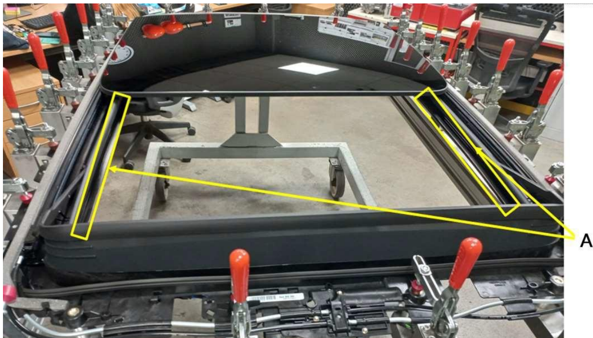
Figure 3 Contamination of roof check
