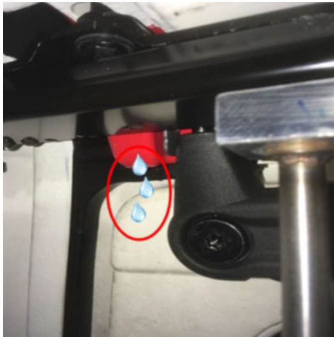
Fig. 2 Water Leak Path Indicating Knuckle Leak
