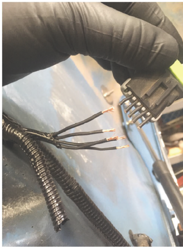
Fig. 4, Splice Pack Removed, Wires Stripped
