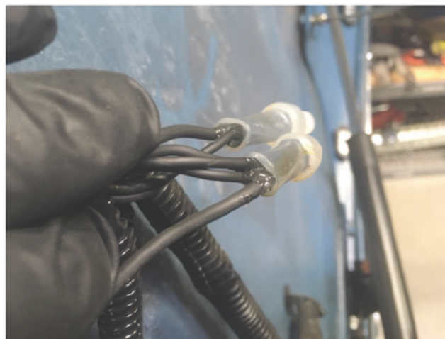
Fig. 5, Wires Sealed with Protective Gel
