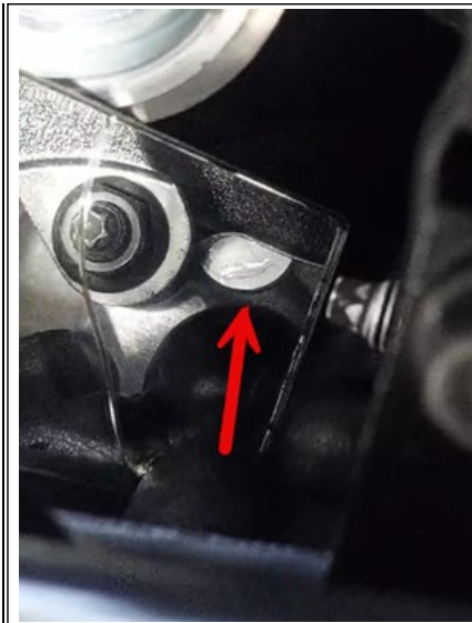
Figure 3 - Using a mirror to inspect between the lower compressor stud and block
