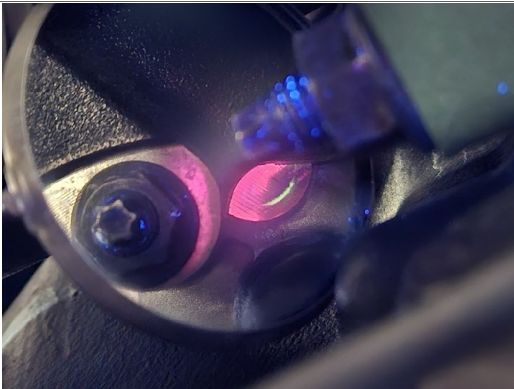
Figure 3 - Using a mirror to inspect between the lower compressor stud and block
