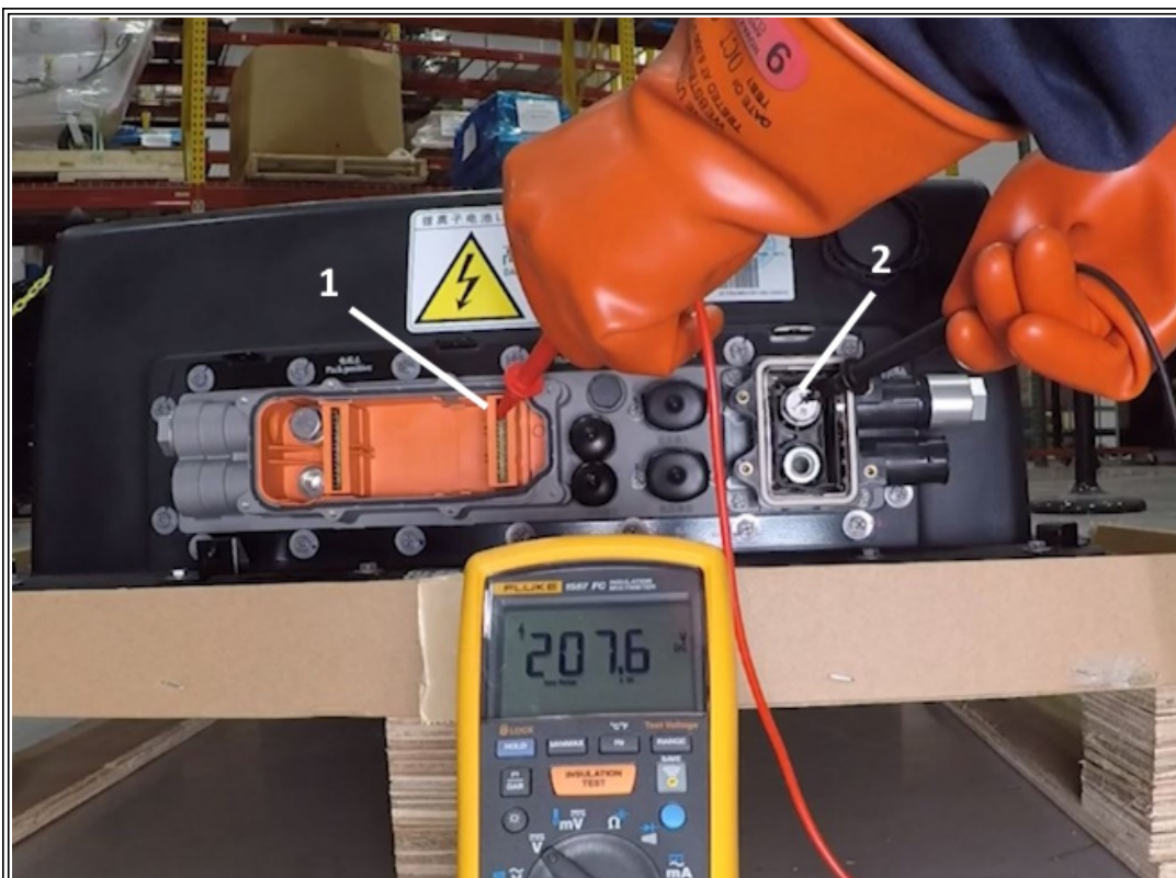
Figure 1: HV Battery Voltage Measurement
