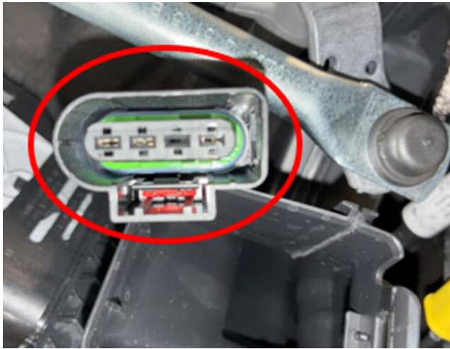
Example image: Female electrical connector contacts on the wiper motor
