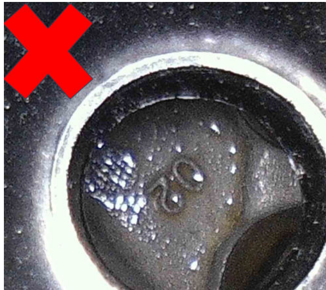
Fig. 4 Umbrella Valve Seal - Missing
