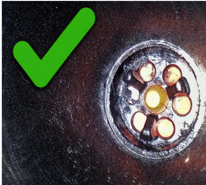
Fig. 5 Umbrella Valve Seal - Present
