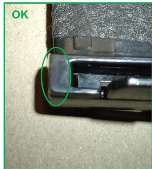
Figure 4 Damage of the sunroof blind slide shoes due to contamination check
