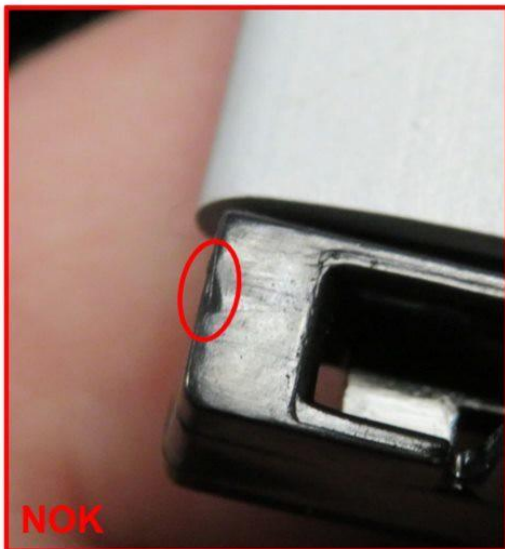
Figure 4 Damage of the sunroof blind slide shoes due to contamination check
