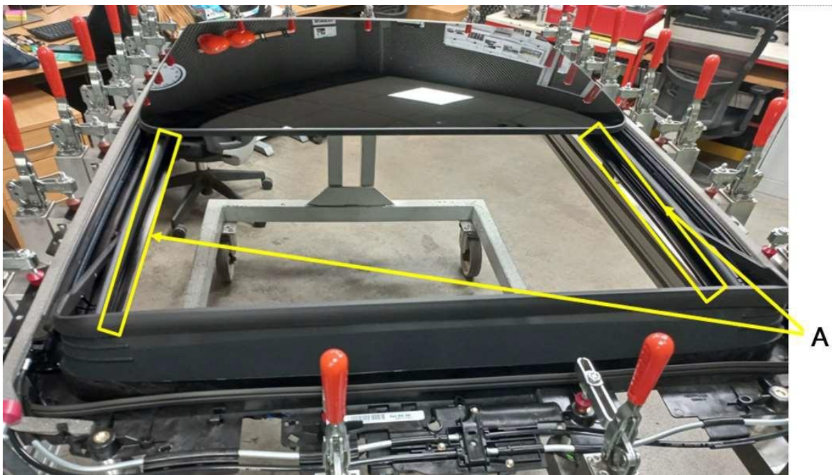
Figure 3 Contamination of roof check
