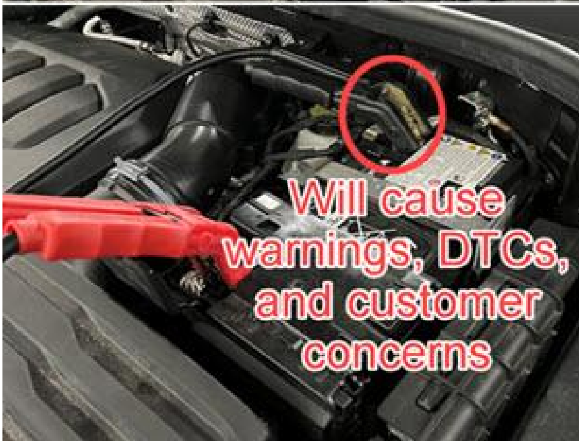
Figure 1. Battery maintainer installation position
