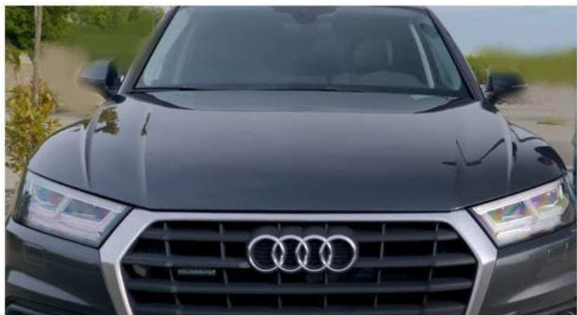
Figure 1: Rainbow-colored shimmer on the inside of lens.
