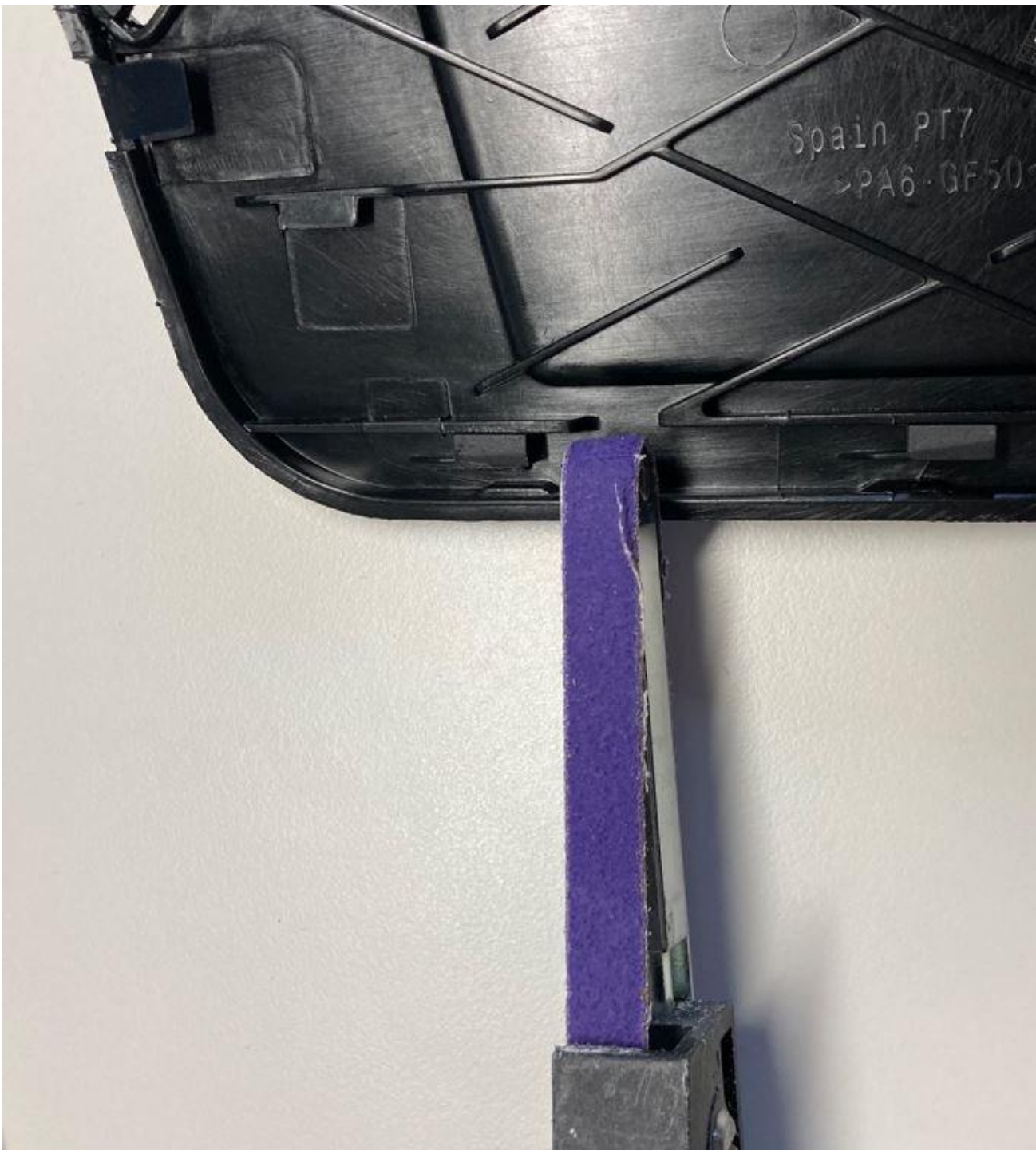
Figure 2. Using a belt grinder to make additional drains.
