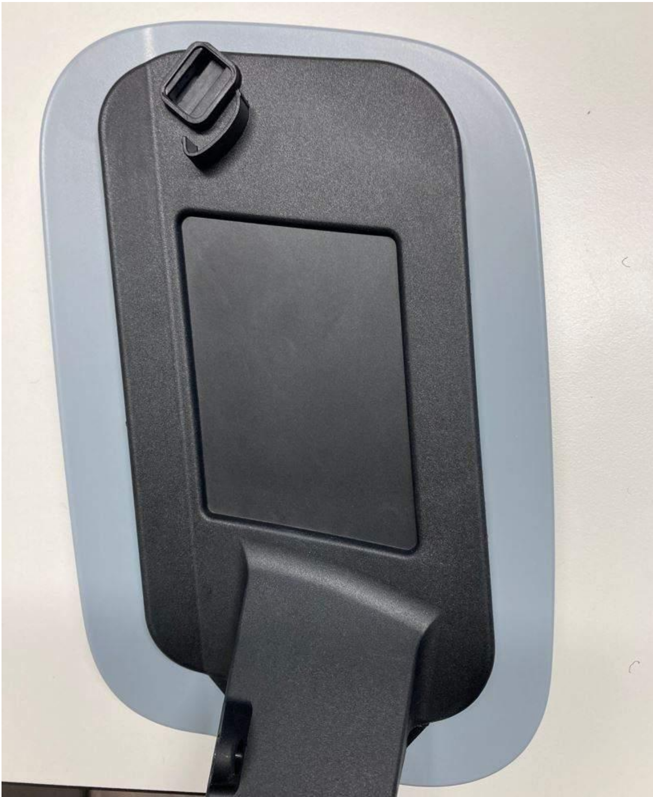
Figure 7. Original fuel filler door installed with excess adhesive removed.
