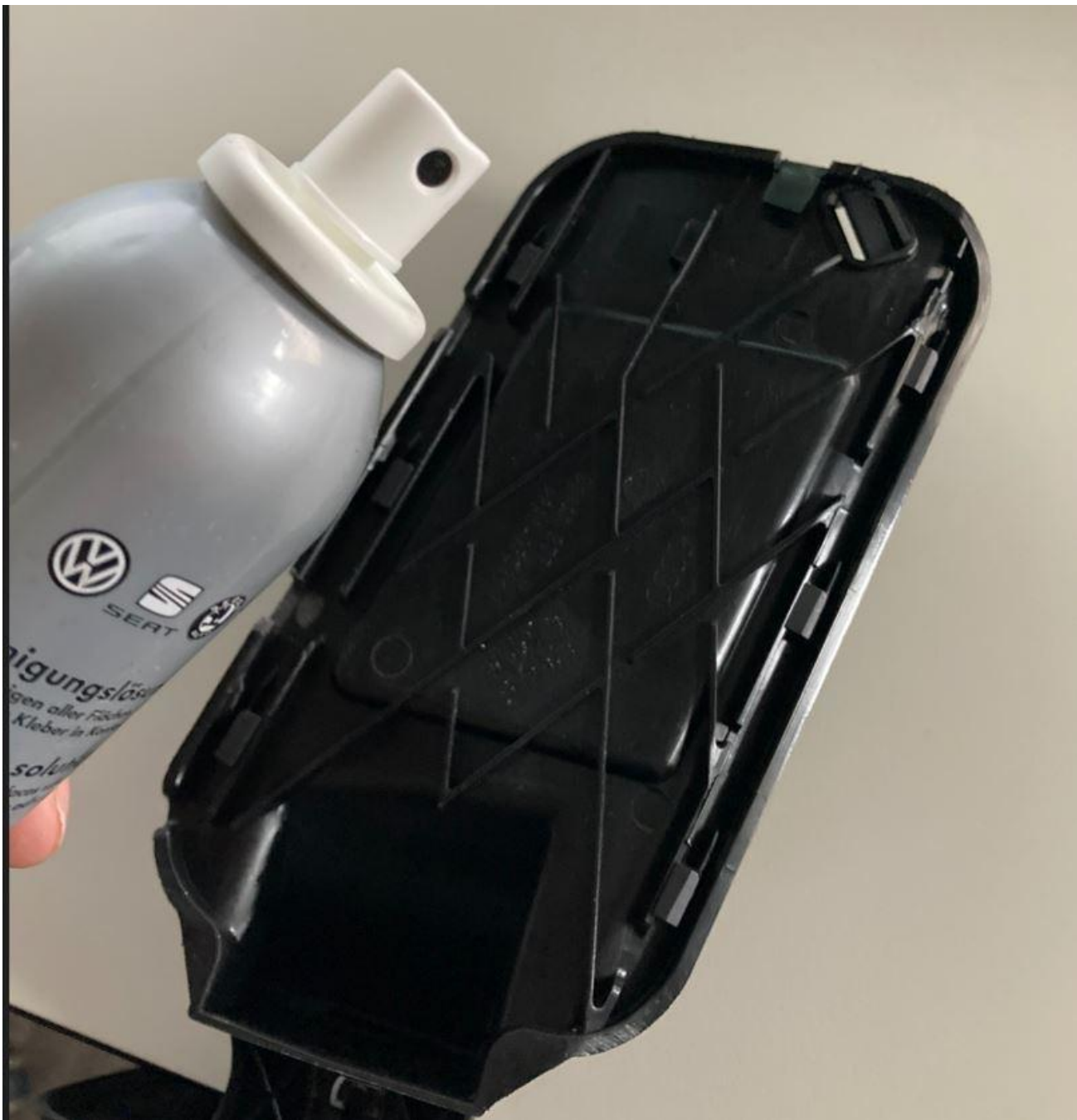
Figure 5. Clean the area which comes into contact with the tank flap as well as the painted reverse side of the tank flap.
