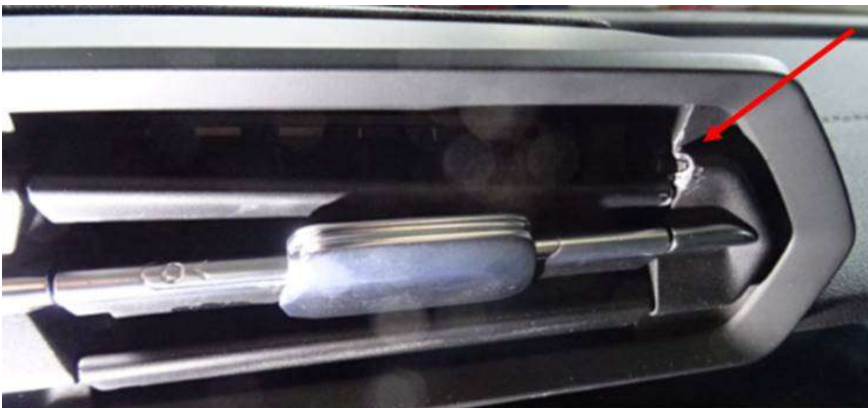
Figure 1. Air vent with broken louver.
