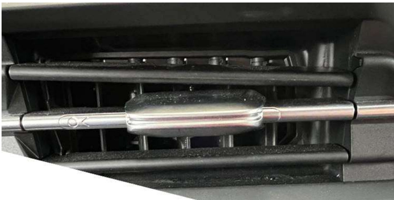
Figure 2. Air vent with broken louver pivot pin.
