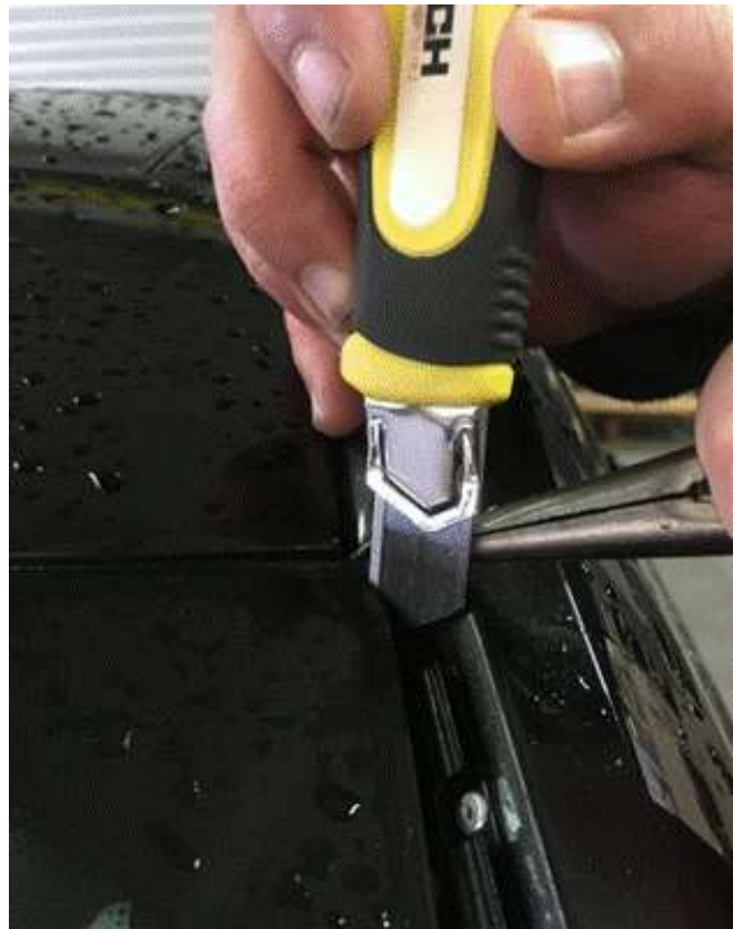
Figure 14. Cutting sealing lip.
