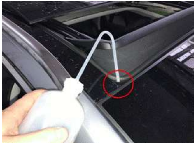
Figure 10. Rinsing the drainage channels.
