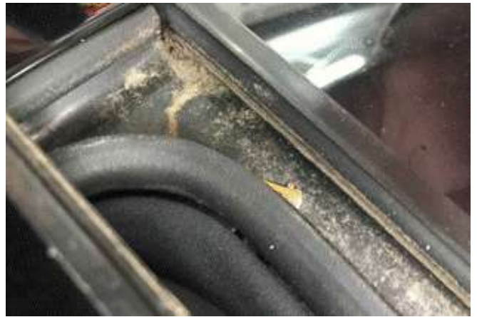
Figure 2. Dirt in the front sunroof frame.
