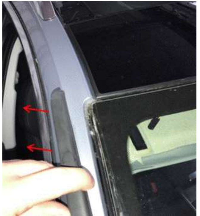
Figure 6. Water deflector removed.
