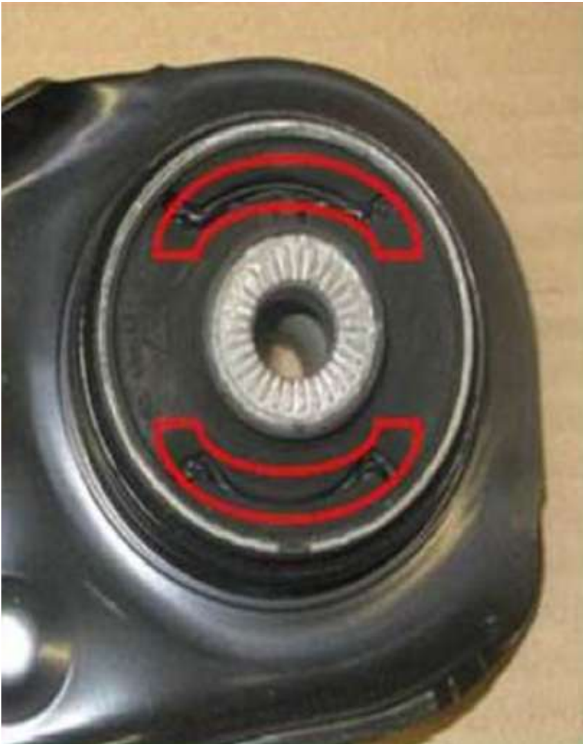
Figure 1. Lithium grease is applied on the red highlighted area.
