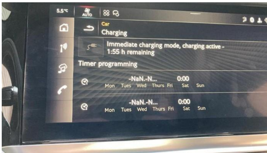
Figure 2. MMI displaying incorrectly set charge timers
