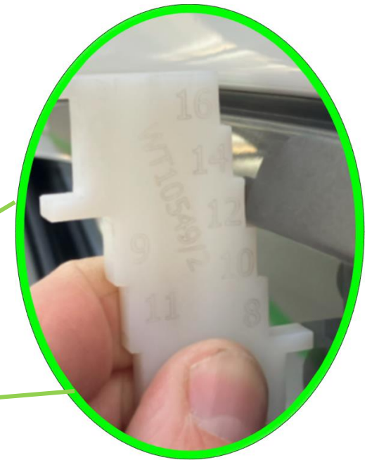
Record measurement (Profile Tool WT10549/2)
