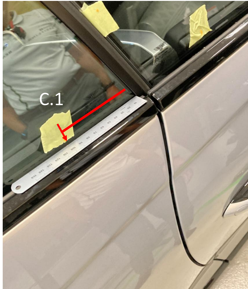
Mark on tape 100mm from div bar (C.1)
