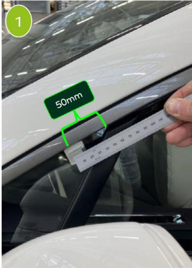
Place block 50mm in front of front div bar
