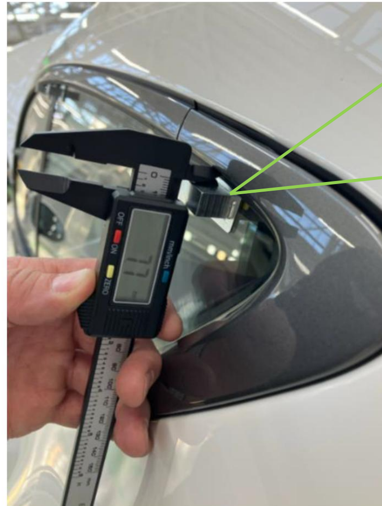
Record measurement for all interlock points
