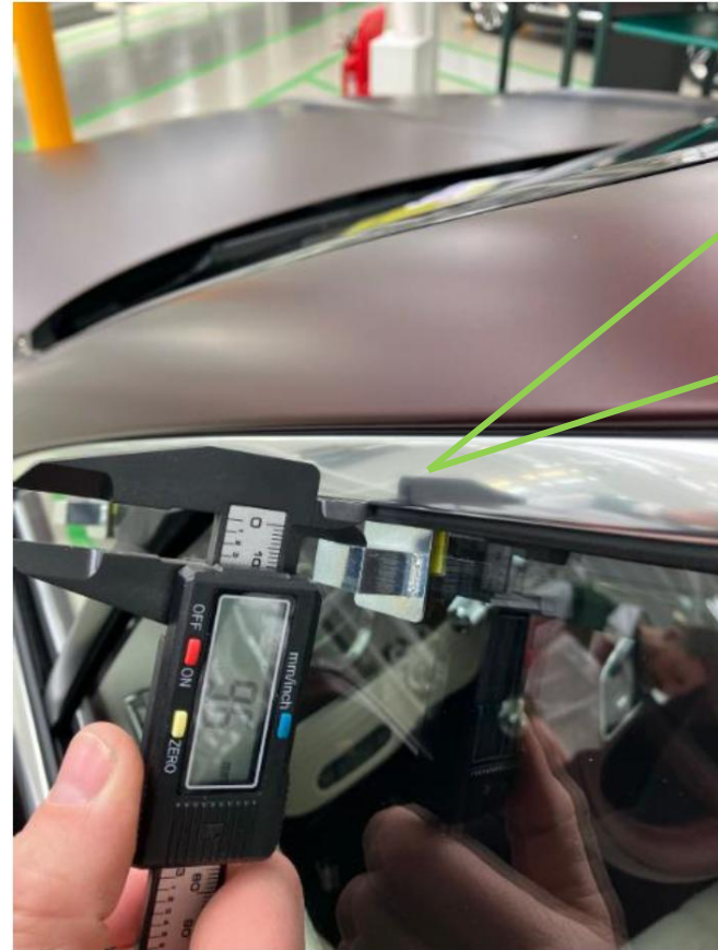
Record measurement for all interlock points
