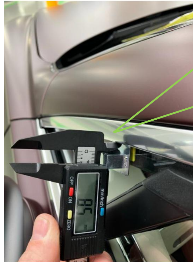
Record measurement for all interlock points
