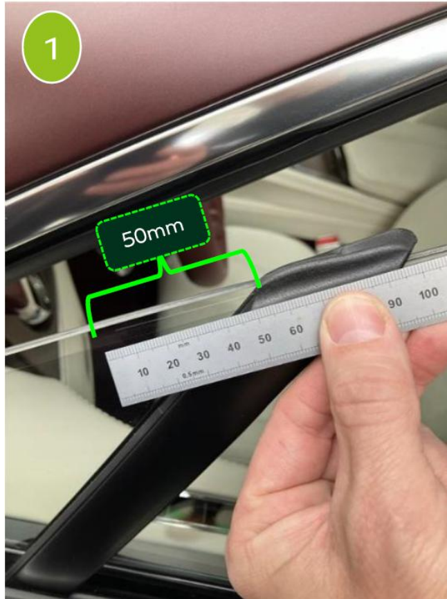
Place block 50mm in front of front div bar
