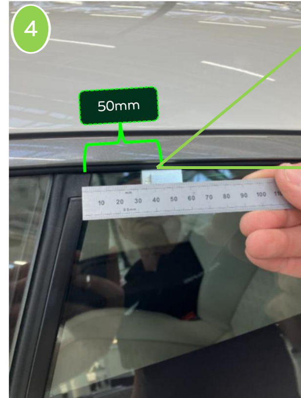
Place block 50mm to rear of rear div bar
