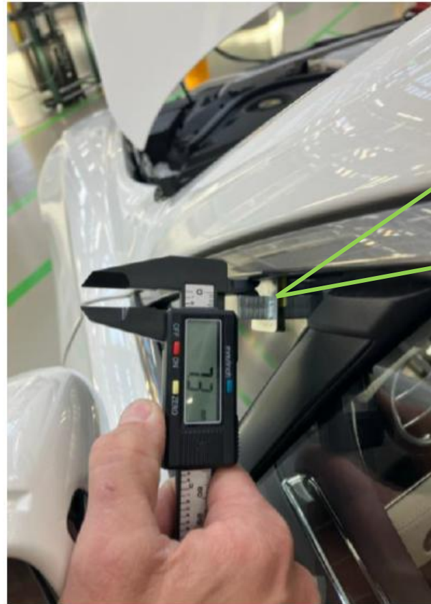
Record measurement for all interlock points
