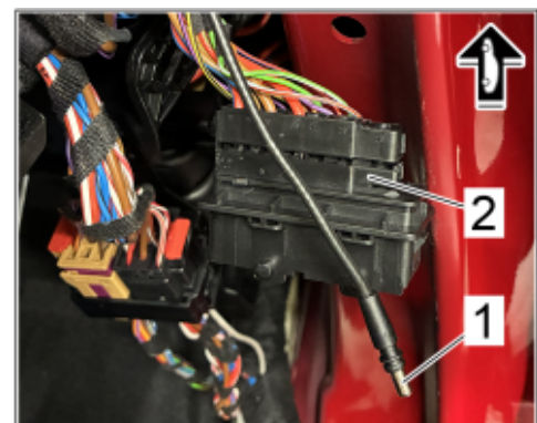
Signal line for door connection point
