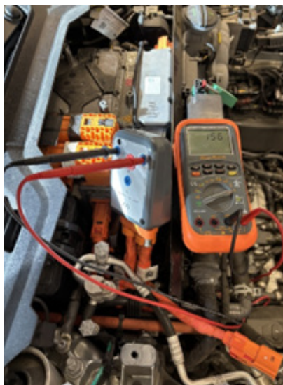
Figure 3 - Measuring Capacitance on Front PE
