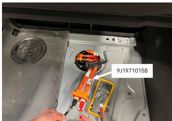
Figure 4 - Measuring Capacitance on Rear PE
