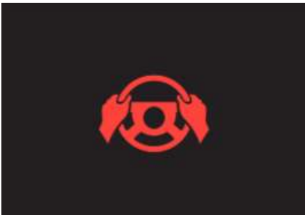
Figure 1. Take over steering warning light.
