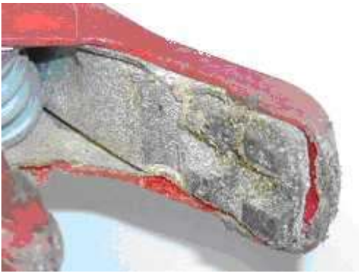
Figure 2. Oxidation on contact surface.
