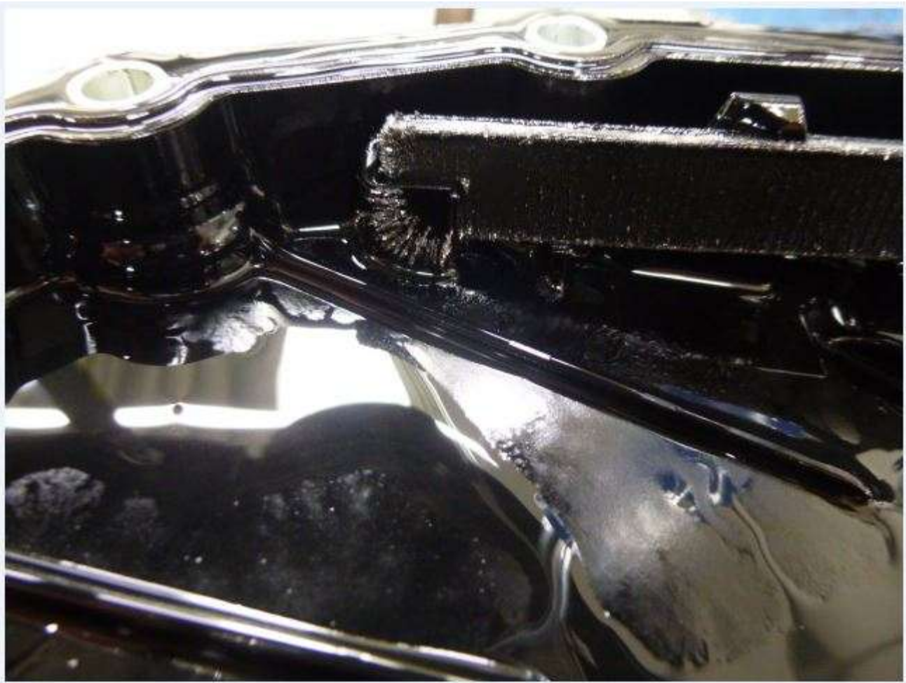
Figure 1. Abrasion is visible on the permanent magnets of the oil pan.
