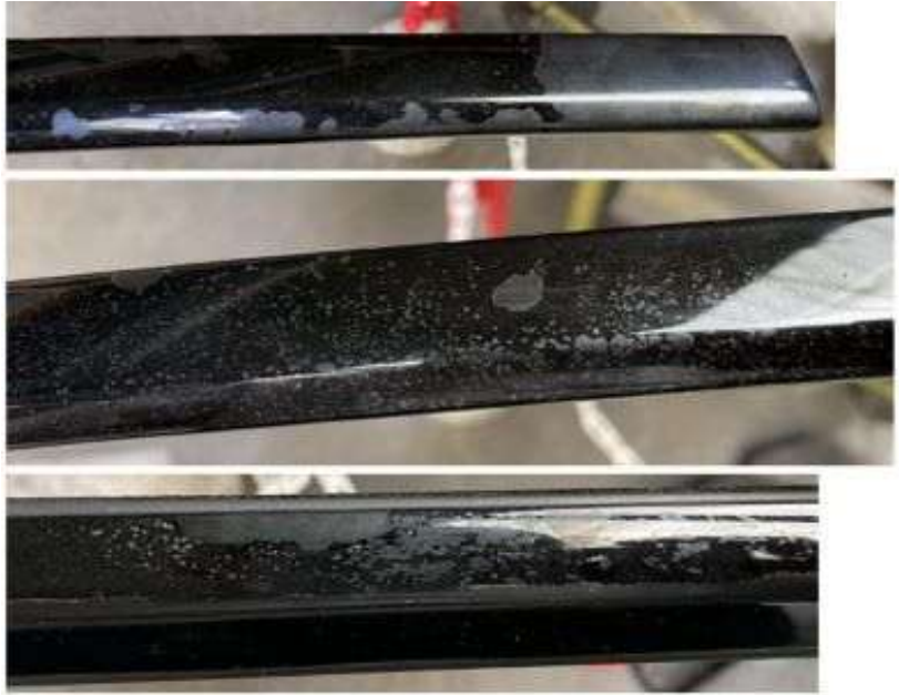
Figure 1. Examples of damage on black trims / trim strips.
