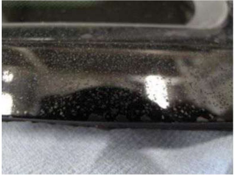
Figure 3. Spots of additional coating.
