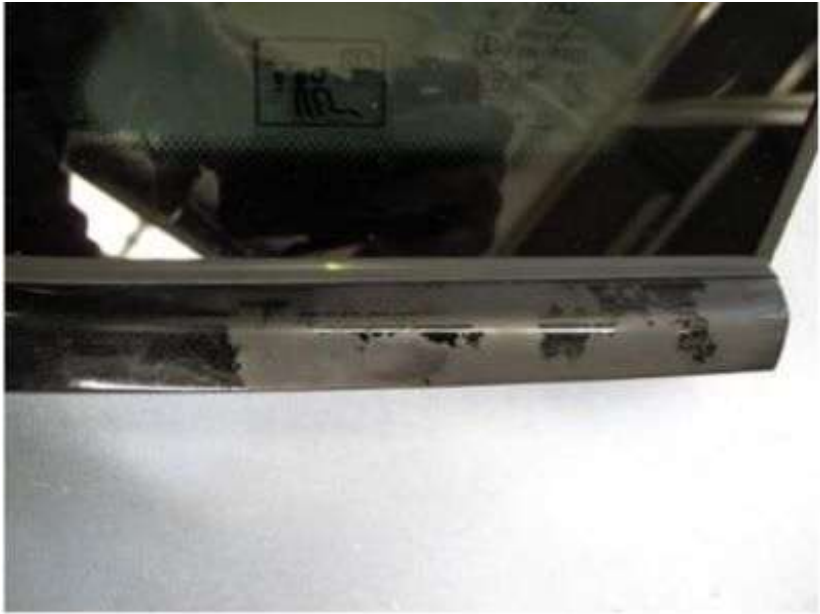
Figure 2. Coat peeled off.
