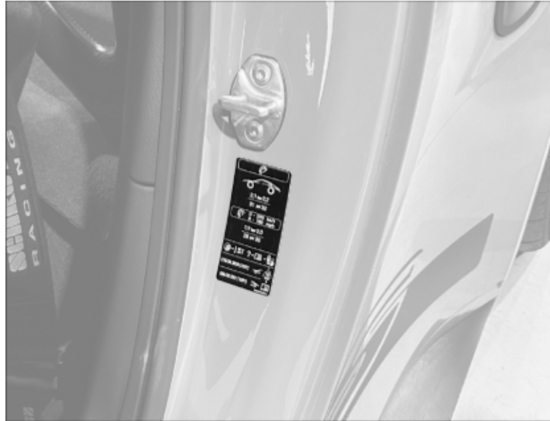
Fitting tire pressure adhesive label
