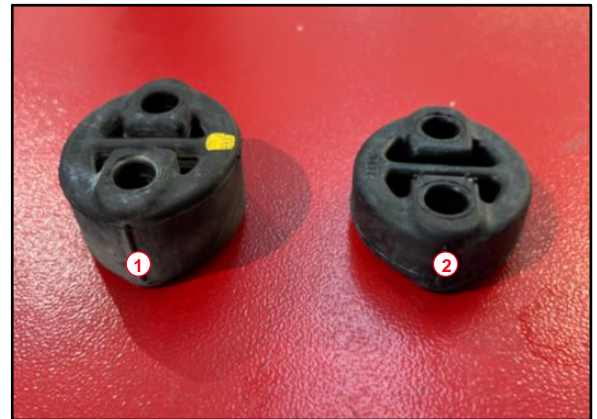
Figure 3. Exhaust Support Hanger 4
