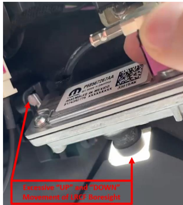
Fig 2 Excessive Displacement of LRCF Boresight OR Insufficient Spring Retention compared to other vehicles OR Excessive Coax Cable Tension
