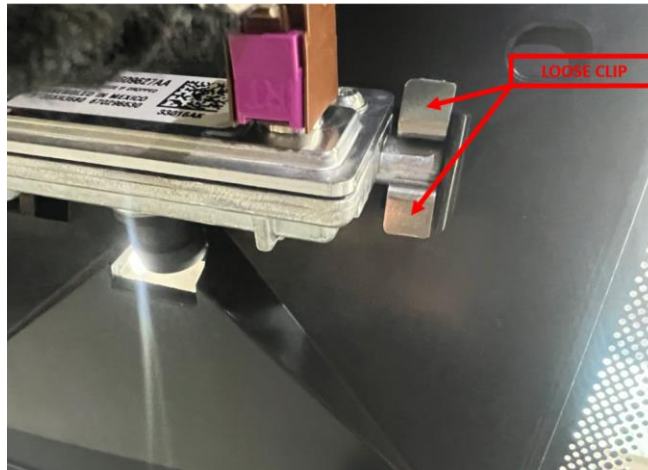
Fig 1 Insufficient Tension of the LRCF Windshield Bracket Mounting Retention Clip
