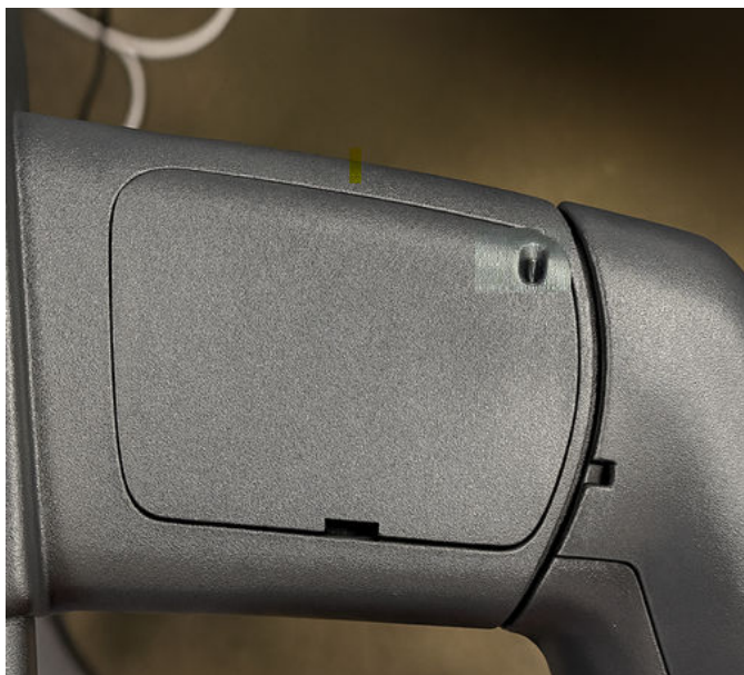
Fig. 10 Properly Installed Mirror Access Cover
