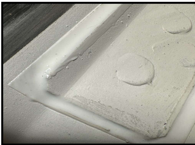
Fig. 14 Apply Seam Sealer
