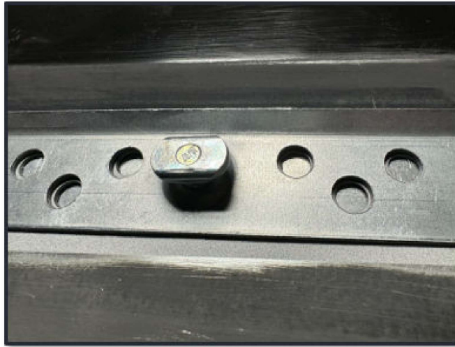
Fig. 11 Roof Rail Bracket Alignment
