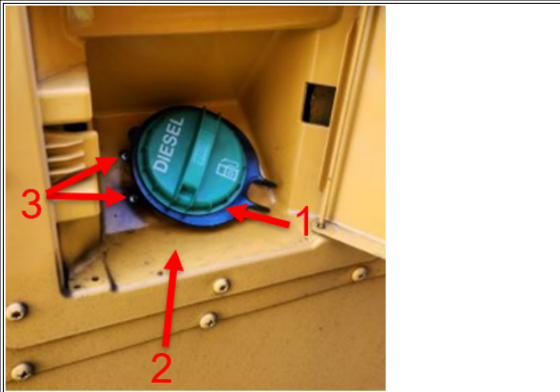
Figure # 1: Fuel Cap Leaking
