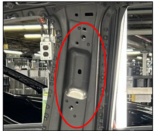
Figure 2. Top of B-pillar to Adjuster Assembly, Front Shoulder Belt Anchor without Trim
