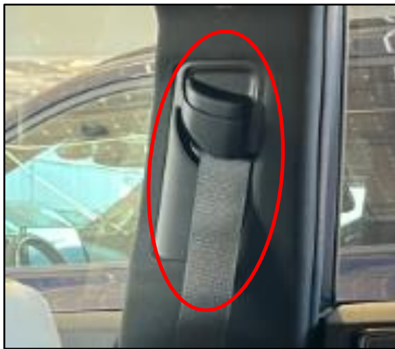
Figure 1. Top of B-pillar to Adjuster Assembly, Front Shoulder Belt Anchor with Trim
