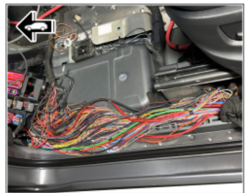
Exposed main wire harness in the passenger compartment, front left.
