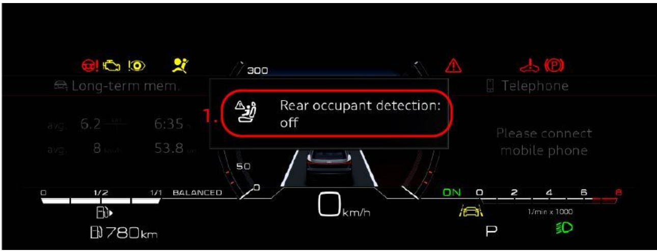
Figure 3. The message above will appear for a few seconds after the ignition is turned on once the rear occupant detection has been turned off.
