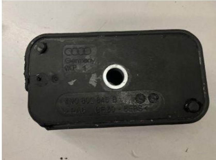
Figure 1. A damaged jacking point leads to water accumulating in the door sill.
