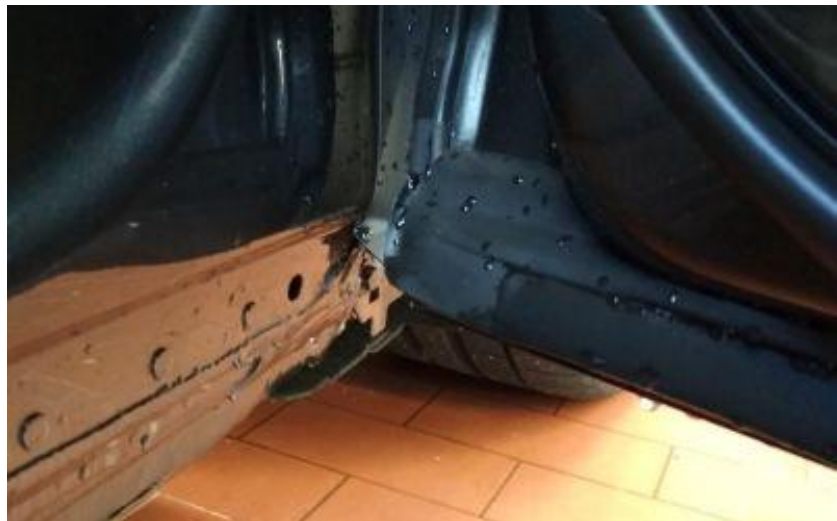
Figure 2. Hole for side clip on door sill trim (example).
