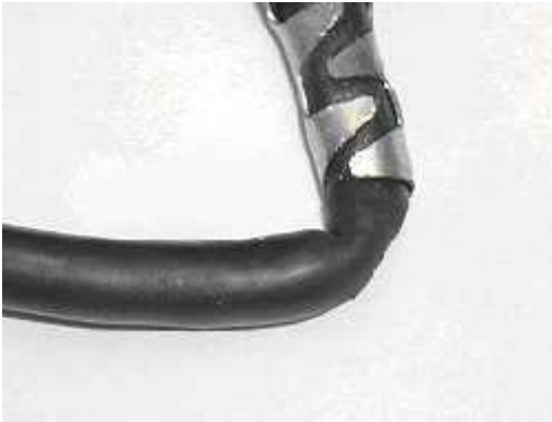
Figure 3. Copper core cracked.
