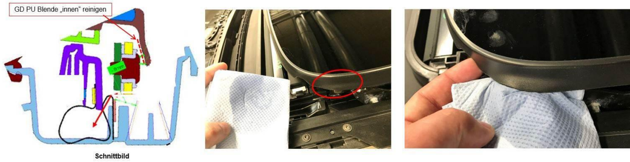
Figure 20. Clen the inside of the glass panel with cleaning solution.
