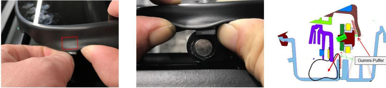
Figure 23. Attach the rubber buffers to the trim.
