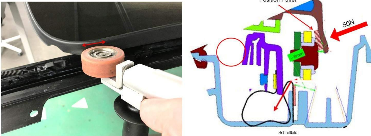
Figure 24. Press down on the rubber buffers.
