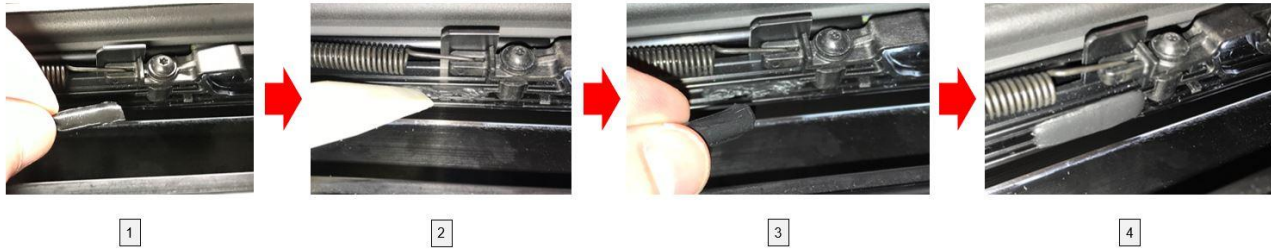
Figure 31. The guide rail channel must be filled with butyl.
