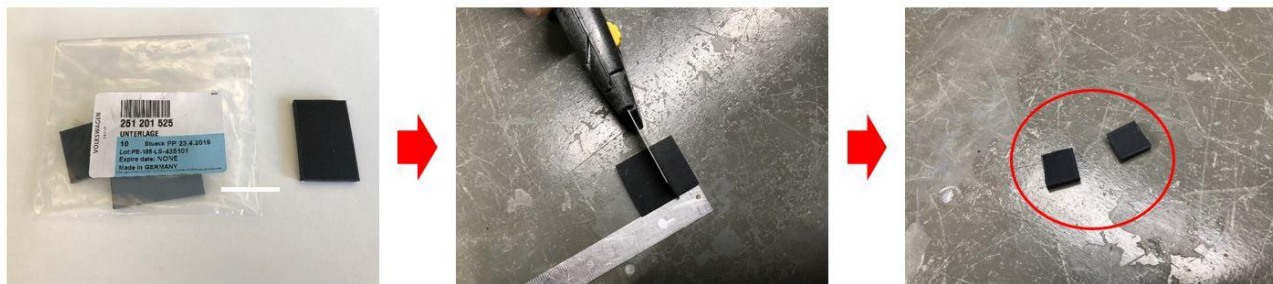
Figure 22. Cut the rubber buffer to size.
