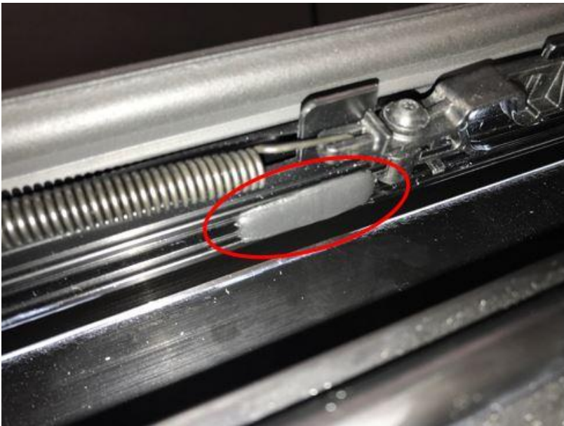
Figure 29. Apply the butyl barrier into the guide rail channel.
