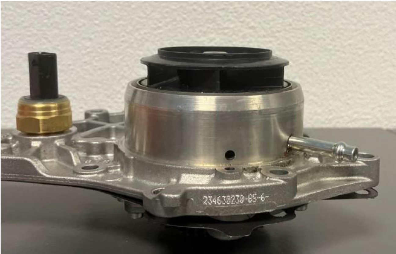
Figure 3. Modulating piston moved back correctly (starting position, not actuated)
