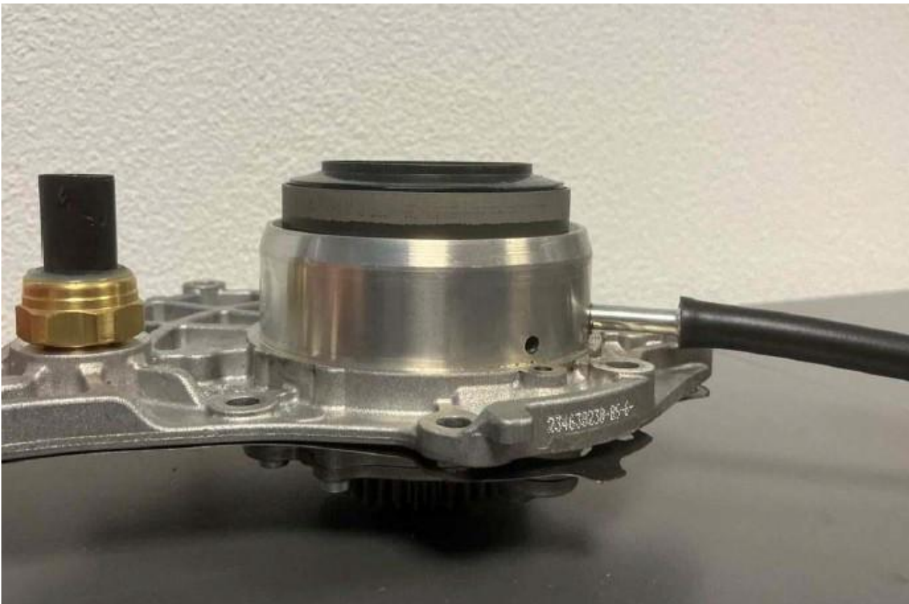
Figure 4. Modulating piston correctly deployed (end position, actuated)
